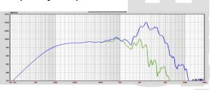
Infinite baffle sound pressure response recorded at 2.83V at one meter.
